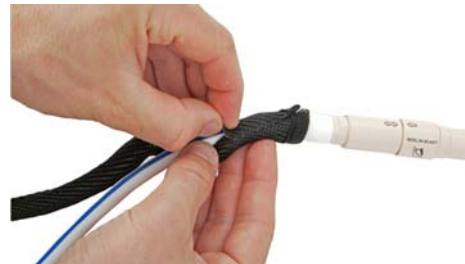
Fig. 5-11 Attaching the cable protector
