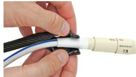
Fig. 5-10 Cable protector on the kink protection sleeve
