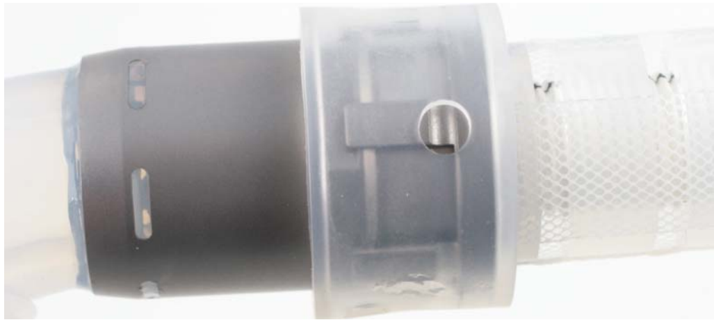
Fig. 7-30 Positioning the silicone cover
