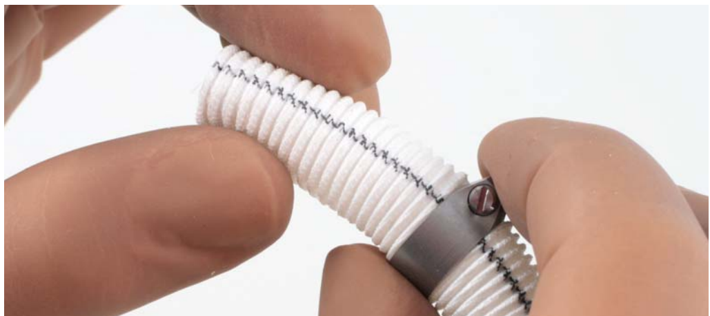
Fig. 7-12 Slide the screw clip down by about 4 cm
