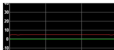
Fig. 7-57 Pressure difference curve before offset correction
