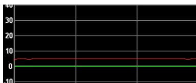
Fig. 6-25 Pressure difference curve before offset correction
