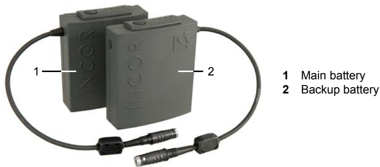
Fig. 4-11 Main battery and backup battery
