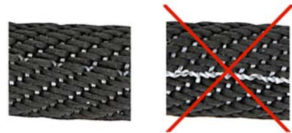
Fig. 5-12 Close-up - cable protector in place
