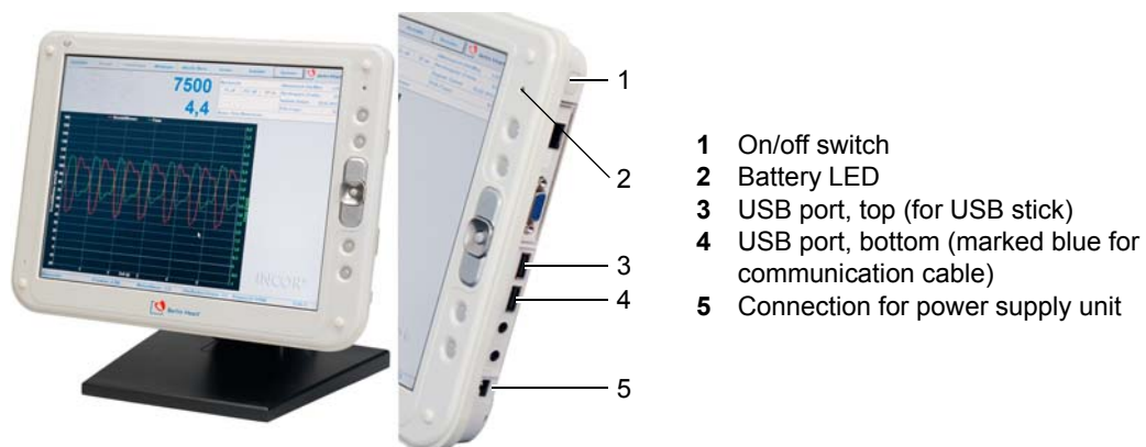
Fig. 6-1 Overview of operator terminal
