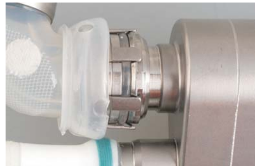
Fig. 7-32 Snap-in connector closed
